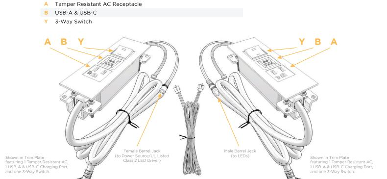
13 ft Connection Wire (connects the two outlets together)
